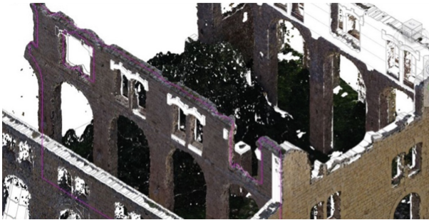
Fig. 2. Visualization of the BIM modelling of walls of the Fornace Penna over its point cloud.
