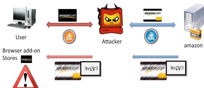
Fig. 2. Workflow illustrating how the MITM attack between the User and Amazon is detected with OBCs
