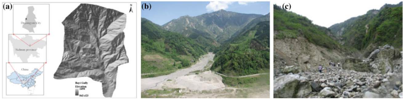
Fig. 1 a The location of Bayi Gully; b full view of the debris flow in Bayi Gully; c loose deposits in the gully
