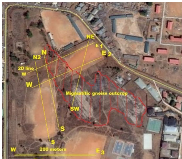
Fig. 2 Satellite imagery of the study area showing 2D electrical resistivity profiles
