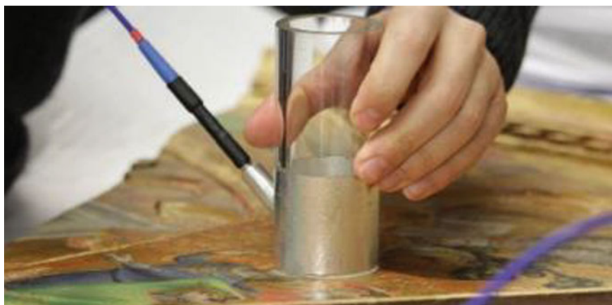
Fig. 6.2 Probe for reflectance measurements with coaxial contactless fibers optics bundle
