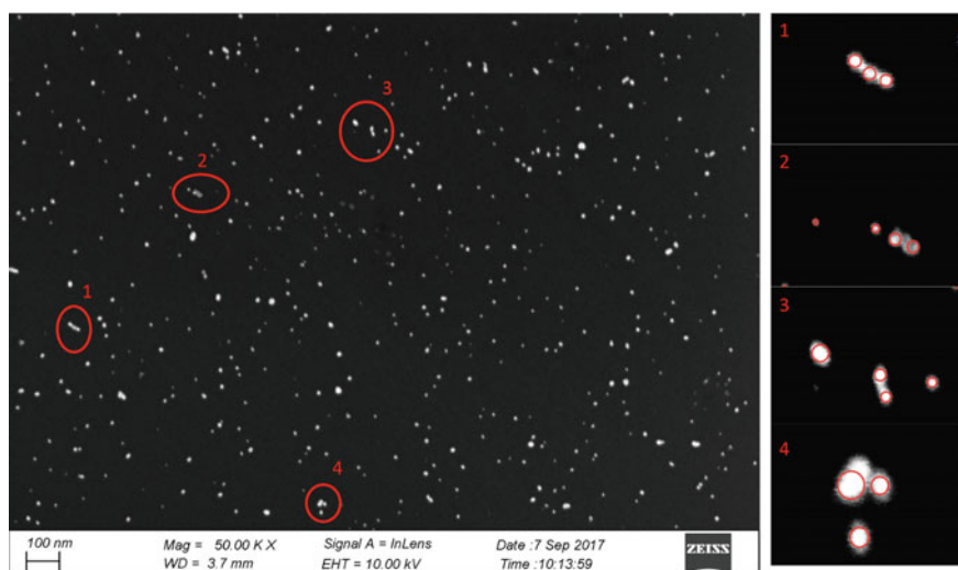
Fig. 7.10 SEM image of Sample 2. On the right, some details of the image with superimposed circle with Hough radius
