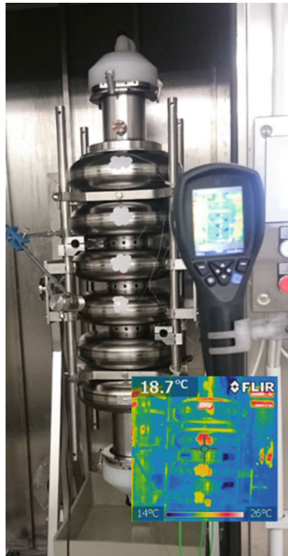
Fig. 25.11 LASA ESS-MB prototype cavity during chemical etching of the RF internal surface via BCP (Buffered Chemical Polishing). The outer surface temperature has been monitored during this treatment by means of an infrared camera (small frame in the bottom)
