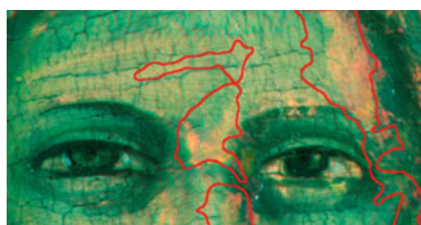
Fig. 6.7 IR false colour image: the XRF image of Cr and Ti (highlighted in red) slightly differs from the IRFC image (clearer in the picture) because the XRF sensitivity for short measuring times
