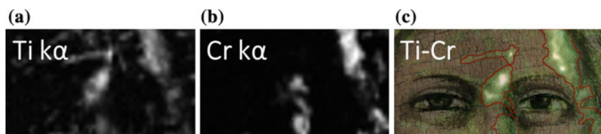
Fig. 6.6 Distribution maps of Ti and Cr (panel (a) and (b) respectively), indicating the restauration regions highlighted in panel (c)
