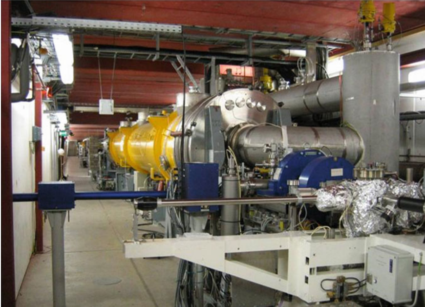
Fig. 24.5 INFN photocathode system connected to the FLASH superconducting accelerator in DESY Hamburg
