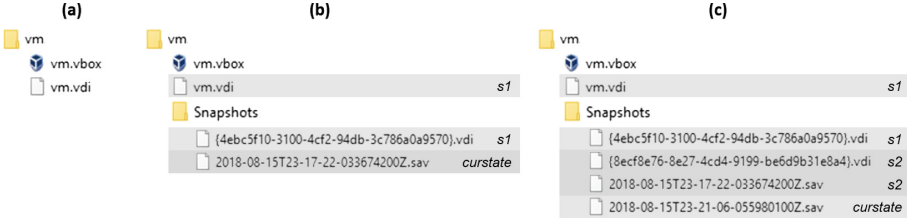
Fig. 4. Evolution of the virtual machine file structure as snapshots are taken
