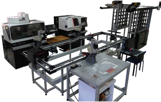
Fig. 7. Case of study: flexible manufacturing cell
