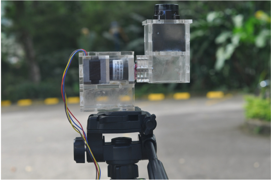
Fig. 2. Configuration of the 3D scanning system based on a 2D LiDAR rotated by a step motor.
