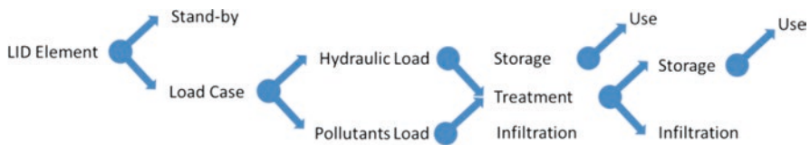
Fig. 9 Operating states and potential features of LID elements in a Sponge City
