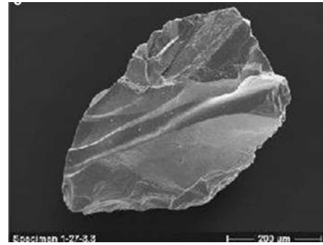
Fig. 2 Severe breakage and abrasion
