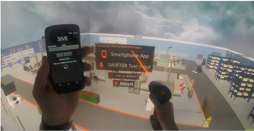
Fig. 7: Creating annotations for smartphone-based communication with the VPI analytics engine.
