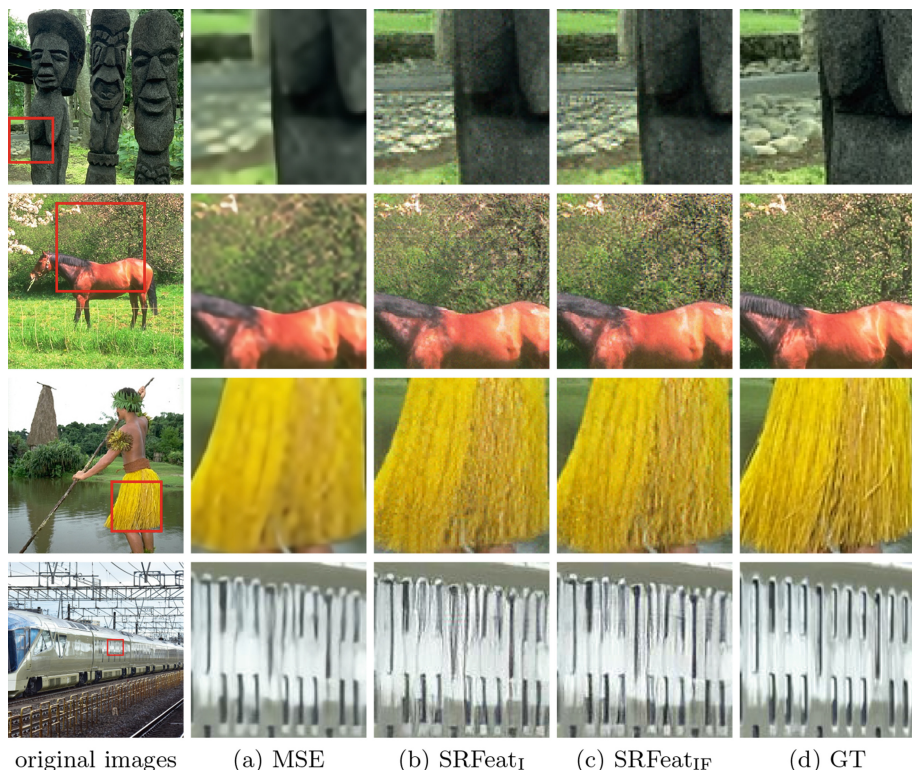
Fig. 5. Qualitative comparison between our models without the feature GAN loss (SRFeat 1 ) and with the feature GAN loss (SRFeat IF ). In all examples, SRFeat IF generates more realistic textures than SRFeat 1 while suppressing arbitrary high-frequency artifacts.
