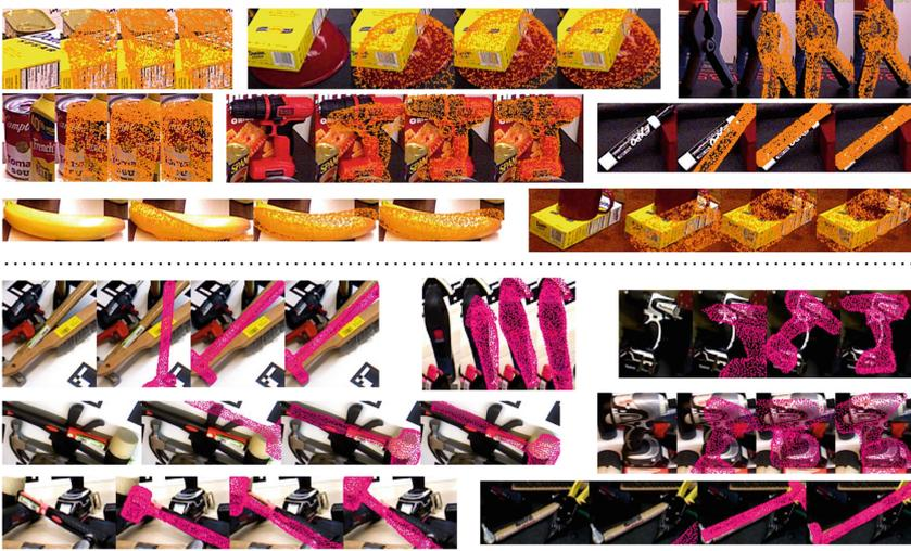
**Fig. 4.** Illustration of pose estimation results by MCN on YCB-Video (upper) and JHUScene-50 (bottom). The projected object mesh points that are transformed by pose estimates are highlighted by orange (YCB-Video) and pink (JHUScene-50). From left to right of each data, we show original ROI, MCN estimates on RGB, MCN estimates on RGB-D and MV5-MCN estimates on RGB-D. (color figure online)
