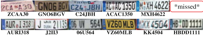
Fig. 8. Detected/unwarped LPs from images in Fig. 1 and final ALPR results.
