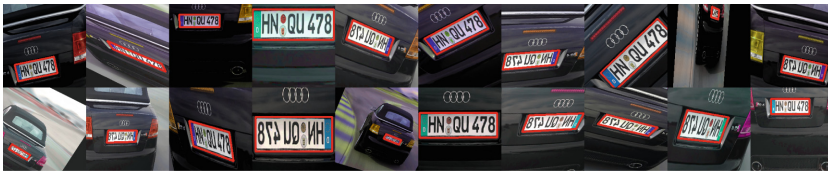
Fig. 6. Different augmentations for the same sample. The red quadrilateral represents the transformed LP annotation. (Color figure online)
