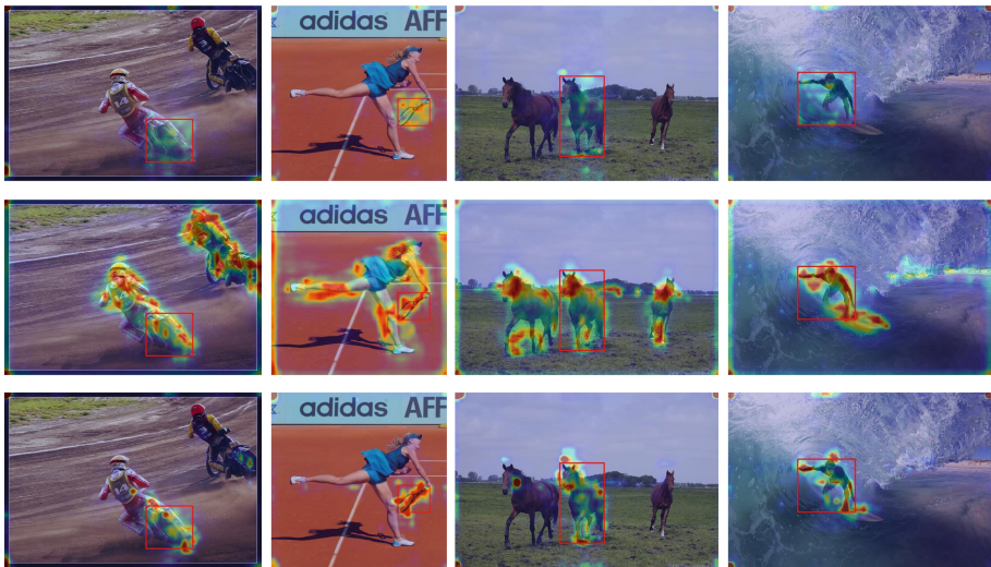
(b) Example results of geometric weights ( top ), appearance weights ( median ) and final weights ( bottom ).
