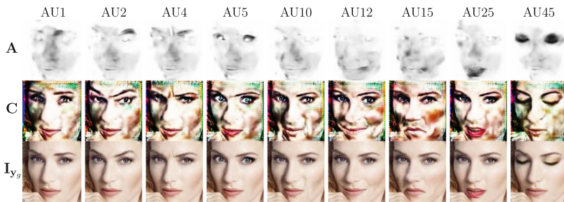
Fig. 5. Attention model. Details of the intermediate attention mask A (first row) and the color mask C (second row). The bottom row images are the synthesized expressions. Darker regions of the attention mask A show those areas of the image more relevant for each specific AU. Brighter areas are retained from the original image.
