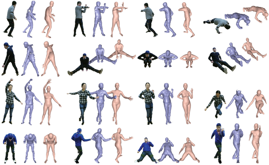
Fig. 5. Example results reconstructed by our system. In each grid, the left image is the color reference; the middle one is the fused surface geometry; and the right one is the inner body shape estimated by our system. (Color figure online)
