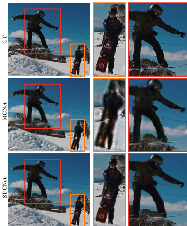
Fig. 6. Comparison of frame prediction methods. Shown from top to bottom are Ground-truth image, MCNet and SDC-Net results. SDCNet is shown to provide crisp and sharp frames, with motion mostly in good alignment with the ground-truth frame. MCNet results on the other hand appear blurry, with artifacts surrounding the persons (framed in red and orange). MCNet results also show checkerboard artifacts near the skis and on the snow background. (Color figure online)
