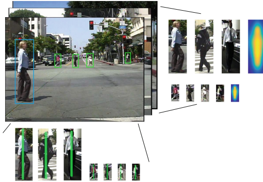
Fig. 1. Pedestrians over different scales could be modeled as a group of 2D Gaussian kernels, indicating that the top-bottom topological line possess high certainty. Our approach attempt to locate this topological line for pedestrian detection.
