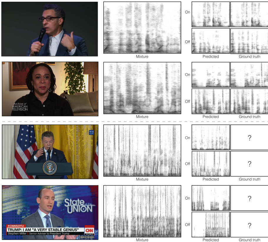
Fig. 7. Qualitative results from our on/off-screen separation model. We show an input frame and spectrogram for two synthetic mixtures from our test set, and two in-the-wild internet videos containing multiple speakers. The first (a male/male mixture) contains more artifacts than the second (a female/male mixture). The third video is a real-world mixture in which a female speaker (simultaneously) translates a male Spanish speaker into English. Finally, we separate the speech of two (male) speakers on a television news show. Although there is no ground truth for these real-world examples, the source separation method qualitatively separates the two voices. Please refer to our webpage ( http://andrewowens.com/multisensory ) for video source separation results.
