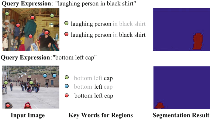
Fig. 6. Visualization of key words for some image regions on the ReferItGame testing. Left to right: input images, key words (black words) for image regions (red, green and blue points), and segmentation results from our full model implemented with VGG16 (Color figure online).
