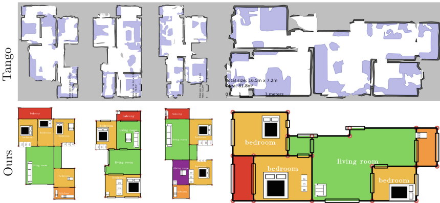
Fig. 7. Comparison against a commercial floorplan generator, Tango Navigator App. Top: floorplan image from Tango. Bottom: our results.
