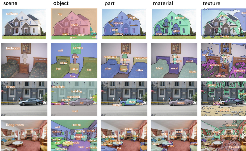
Fig. 5. Predictions on the validation set using UPerNet (ResNet-50). From left to right: scene classification, and object, part, material, and texture parsing.
