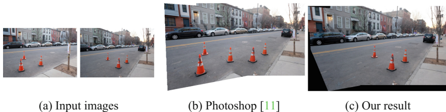
Fig. 3. Motivating example for multiple registrations. State of the art commercial packages like Adobe Photoshop [11] duplicate the traffic cones and other objects.
