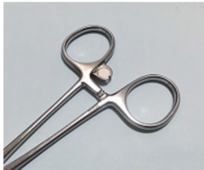
Fig. 1. Surgical instrument with RFID tag [3]
