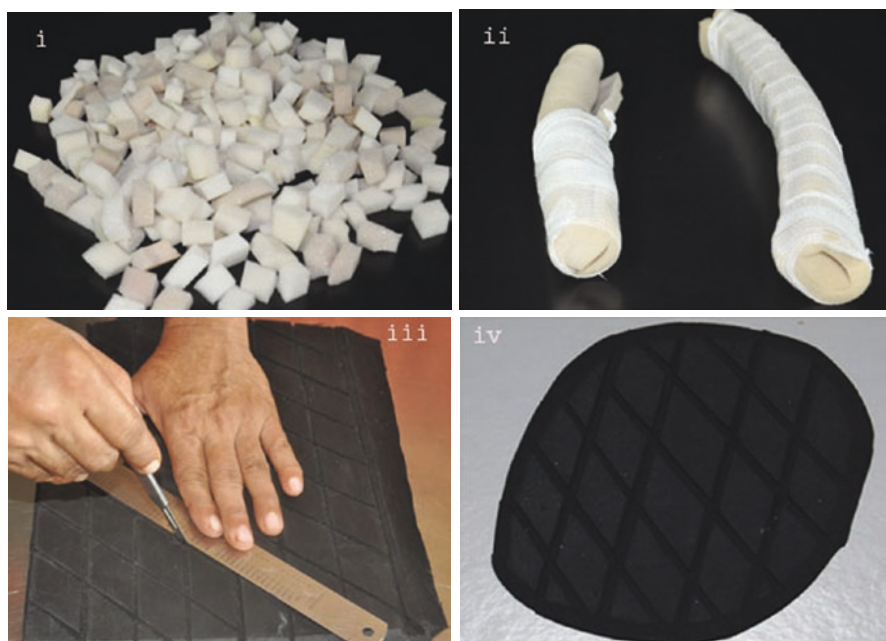
Fig. 9.7 (i) CCF pieces for chalky bag (ii) sandwich mould on right and partially completed sandwich mould on the left (iii) carving diamond shaped grooves on MCR mould to facilitate lymph drainage (iv) Microcellular rubber mould
