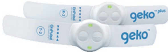
Fig. 10.4 (Geko®, Firstkind Ltd., UK) A neuro muscular electrostimulation (NMES) device. This is applied to the skin behind the knee
