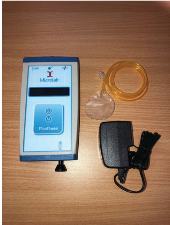
Fig. 10.1 PicoPress® (Medi Group, Australia) pressure transducer which can be left under the bandage allowing for repeated measurement
