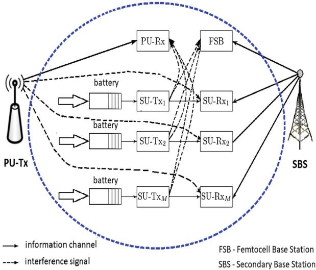
Fig. 1. System model of cognitive femtocell network.
