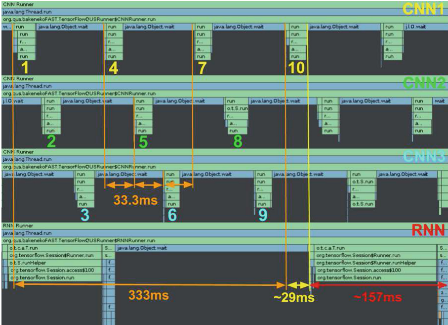
Fig. 6. Timing diagram of the three CNN and one RNN threads. The orange lines show the arrival of the input frames.
