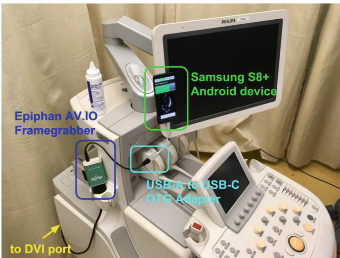
Fig. 1. The physical system setup. The frame grabber connects to the DVI output of the ultrasound machine. It is then connected to an OTG adapter and plugged directly into the Android’s USB-C port.
