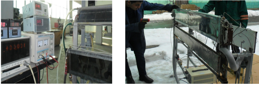
Fig. 6 Test bench for determining heat losses in flat channels of pv modules
