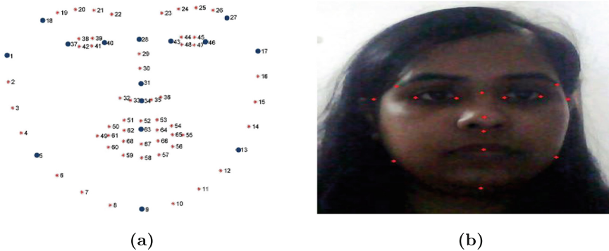
Fig. 7: Points (a) used to estimate head pose (marked with blue dots) and (b) detected by our system
