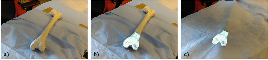
Fig. 3. Since {}^S\mathbf{T}_V(t) is known, the real object in (a) is overlaid with the rendered volume shown in (b). Correct overlay persists even if the real object is covered in (c).
