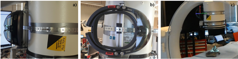
Fig. 2. The prototype uses a Microsoft HoloLens as tracker which is rigidly mounted on the C-arm detector, as demonstrated in Fig. (a) and (b). In (c), the coordinate axis of the RGB tracker is shown in relation to the mobile C-arm.
