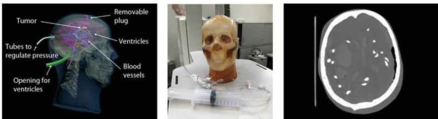
Fig. 1. The CAD model of the phantom, the experiment setting and an example slice of CBCT acquisition of the phantom are shown from left to right.
