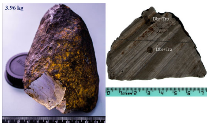
Fig. 1 The general view of the Uakit meteorite (IIAB) and a cut-off with troilite-daubreelite nodules. Symbols: Dbr+Tro – troilite-daubreelite nodule
