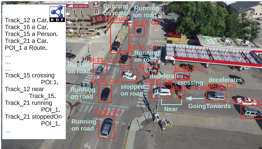
Fig. 4. Situation understanding: spatio/temporal relations among people and vehicles, together with high-level events are detected through ontology reasoning
