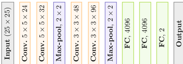
Fig. 1. Architecture of the CNN model used for brain extraction
