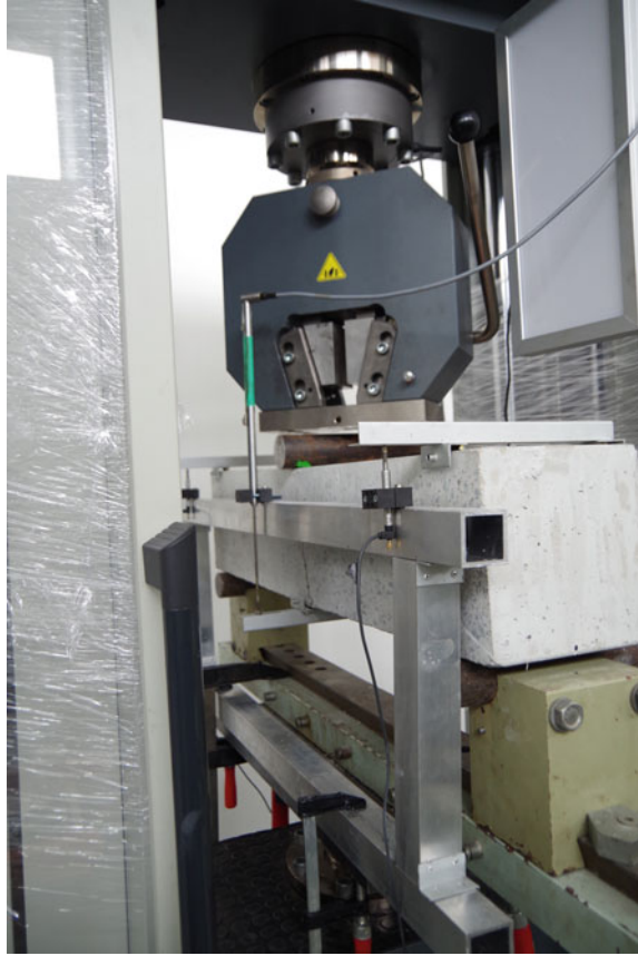
Fig. 7 Photo of the bending test showing a beam sample in the testing machine with the frame for displacement measurements and displacement sensors
