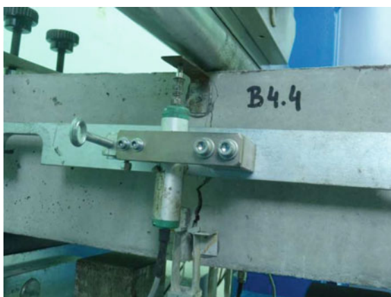
Fig. 1 A prismatic specimen with a notch during the flexural test (LOP method)
