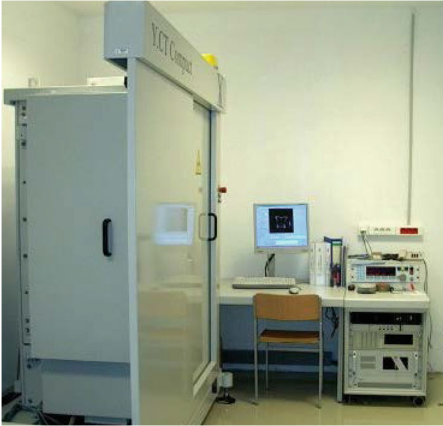
Fig. 1 CT-Scan: YXlon COMPACT with a YXlon tube of 225 kV/30mA at University of Burgos (Spain)
