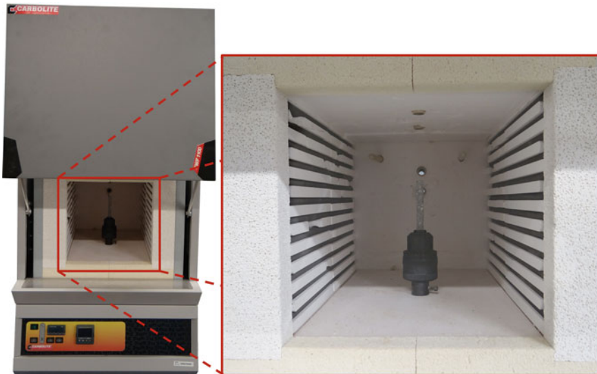
Fig. 2 Electrical furnace containing a typical clamped specimen
