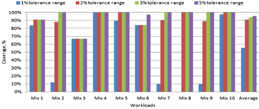
Fig. 3. Coverage percentage of cap sizes with peak performance points for various tolerance ranges
