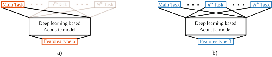
Fig. 2. A hybrid-task learning (HTL) system which adapts its architecture depending of the input features. The same system is represented, where \alpha and \beta are two different kind of input features randomly fed to the system (for instance real and simulated data). (a) As the input features are \alpha type, the HTL system behaves as a single-task learning system. (b) The \beta type features force the system to behave as multi-task learning system with N auxiliary tasks.
