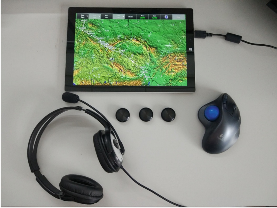
Fig. 5. Hardware used in the flight tests; MS Surface tablet, office headset, and PTC buttons
