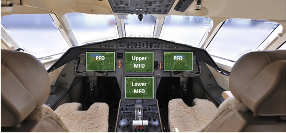
Fig. 1. Position of Primary Functional Display (PFD) and Multi-function Display (MFD) in the cockpit of Falcon F900
