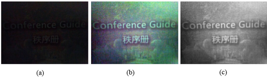
Fig. 4. Fusing two enhanced images for generating a better enhanced image, where (a) is the enhanced image from color space, (b) is the enhanced image from frequency domain and (c) is the enhanced image from the proposed method.
