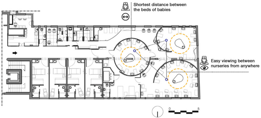
Fig. 9 Diagram showing the shortest distance between nurses and babies. Source: Author's own illustration (2016)
