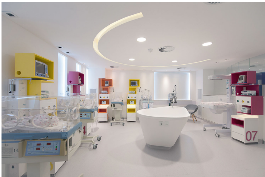
Fig. 12 Smooth surfaces avoiding contamination and corners
