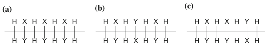
Fig. 2.3 Fischer projections for polymer chain with different structures: a isotactic, b syndiotactic, c atactic
