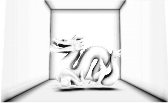
Fig. 1. Map of occlusion shadows generated by the normal-oriented hemisphere SSAO technique.
