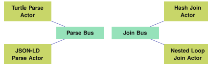
Fig. 2. An example of two different buses each having two subscribed actors. The left bus has different actors for parsing triples in a certain RDF serialization to triple objects. The right bus has actors that join query bindings together in a certain way.
