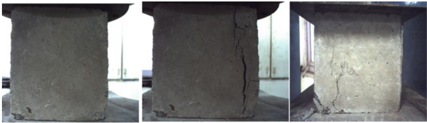
Fig. 1 Sample image of concrete cube with and without crack
