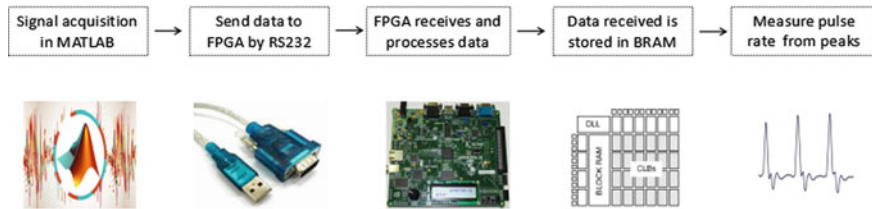
Fig. 3 Block diagram for FPGA implementation of the techniques
