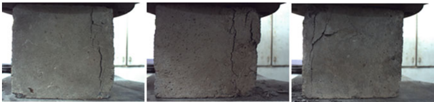
Fig. 3 Sample concrete crack images
