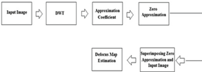
Fig. 3 Block diagram for defocus map using modification of approximation by edge projection
