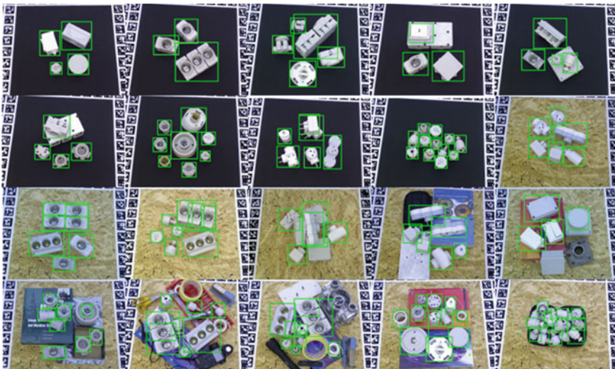
Fig. 2 Recognition result of the instance segmentation network
