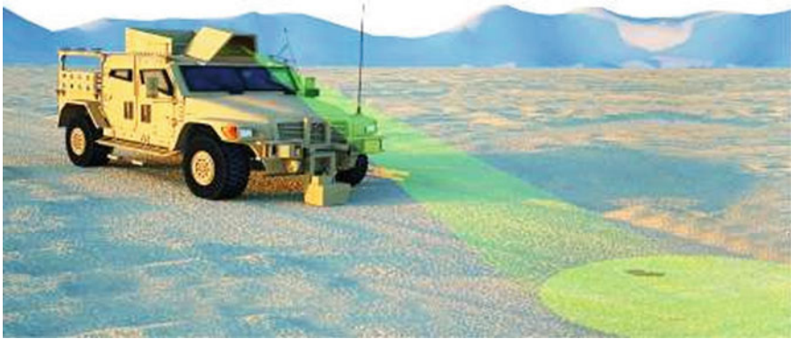
Fig. 2 Military vehicle to detect IED using LIBS
