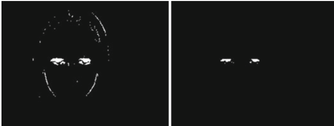
Fig. 6 Threshold difference image prior to erosion (left), and same image after erosion (right). Erosion removes noise caused by insignificant motion in the scene
