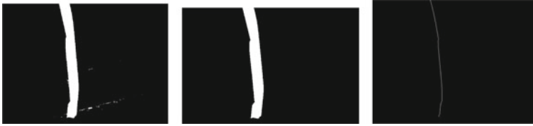
Fig. 3 Binary image before and after noise removal and skeletonized version
