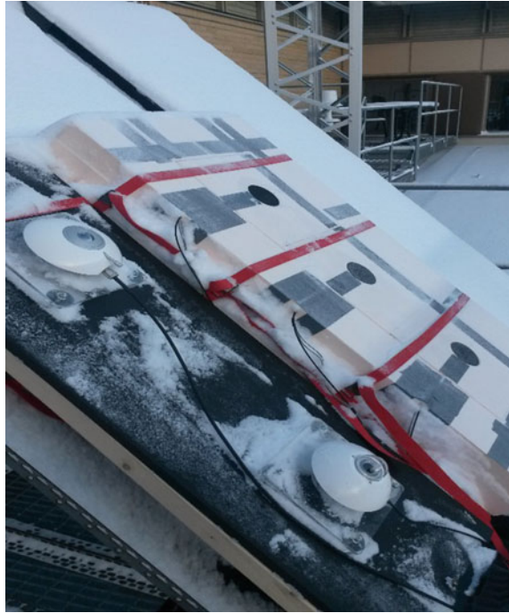
Fig. 3 Experimental setup. Three SAT units shown as black circle areas to the right in the figure, with SAT1 (heated) at the top and SAT0 (unheated) at the middle position). (The third SAT shown was not used in this work.) To the left side, the pyrgeometer (top) and the pyranometer (bottom) are seen
