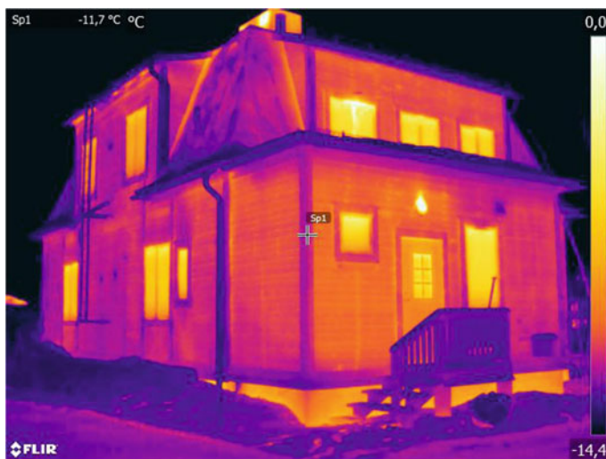
Fig. 6 Infrared image of house B52 from outside. The poor thermal performances of many components of the building envelope are clear. Outdoor temperature: -13\text{ }^{\circ}\text{C}
