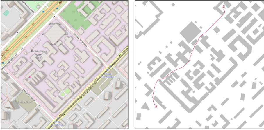
Fig. 5. Left: Map fragment of an urban environment retrieved from OpenStreetMaps. Right: An example of a task, solved by eLIAN on the corresponding grid.
