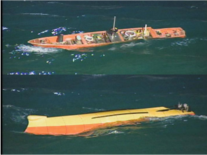
Fig. 28.1 View of model 5514 during capsizing testing in MASK basin
