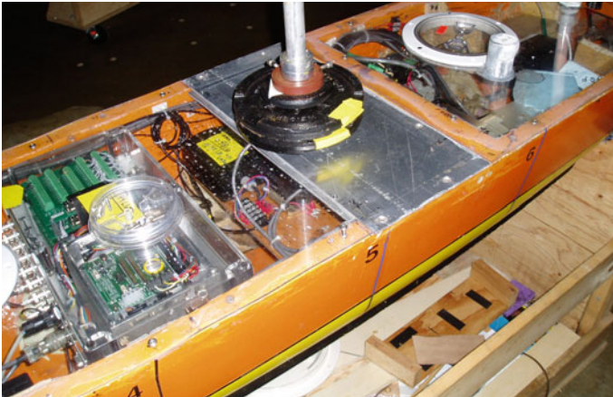
Fig. 28.3 Midship OBC, GM pole, and instruments
