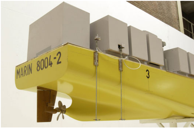
Fig. 37.3 Stern-quartering view of MARIN Model 8004-2 showing rudder and propeller (MARIN 2009)
