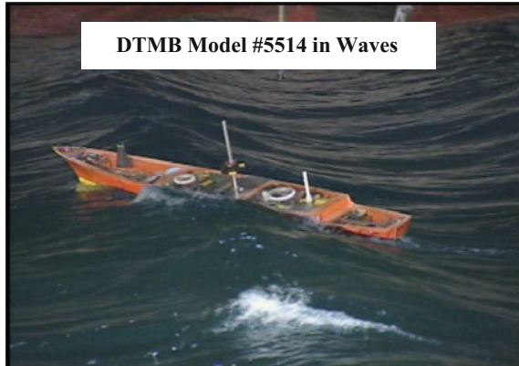
Fig. 30.1 Experimental testing of ship performance in heavy seas using regular waves
