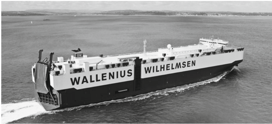
Fig. 10.1 The Panamax pure car and truck carrier that serves as case vessel in this paper
