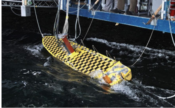
Fig. 12.1 High roll motion without capsize and very low amount of green water in stern quartering seas
