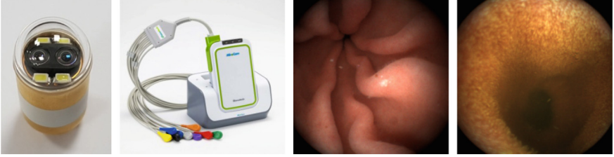
Fig. 1. Stereo-type wireless endoscopic capsule, wireless receiver, and captured images in the stomach and the small bowel, from the left.
