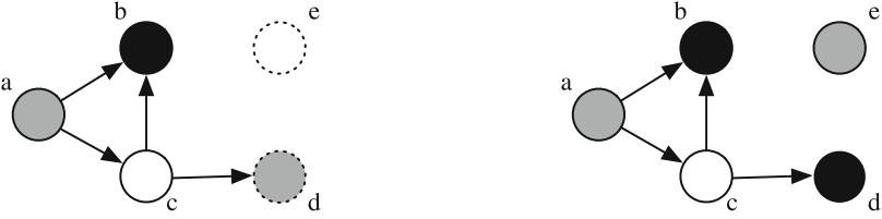
Fig. 1. In this figure, we illustrate the coloring of an arbitrary graph. (Left): Each node has a unique color, thus five colors are used for coloring five nodes (solid Black, solid Grey, solid White, dashed Grey, dashed White). (Right): This graph can be colored using only 3 colors—is 3-colorable (solid Black, solid Grey, solid White).
